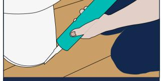
11. For slash areas such as bathrooms, waterproof skirting/scotia/ trims can be used. Cut the flooring around your WC base leaving a 6mm expansion joint. 100% Silicone sealant can be used to fill in the gap. Silicone can be used in small areas such as around sink pedestals but should not be used on large areas as it will restrict the expansion and contraction of the flooring causing the joint edges to fail.
