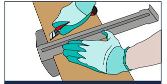
4. To cut your ClickLux planks to size, measure and mark with a pencil. Using a T-square and utility knife, apply pressure and score along the line. Gently flex along the scored edge until it separates into two pieces.
