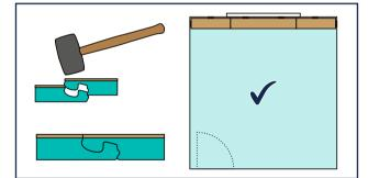
7. To Start the first row, place the planks against the wall and the groove joint facing away from the wall. Align the short edge joints and gently tap into place using a soft rubber mallet. Be sure to align the joints accurately and tap directly in line with the joint to ensure a perfect seal, without damaging the joints. Continue to install further pieces until the first row is complete.
