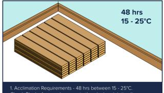
Check Planks for any damages to the plank or jointing lips. Dispose of damaged planks. Read Instruction manual supplied in the box for preparation and in depth advise.
