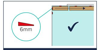
6. Begin installing ClickLux from the left side of your room and always work to the right. Use spacer wedges next to any piece that meets a wall to ensure a 6mm expansion gap is left around the perimeter.
