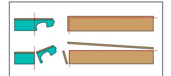
5. To achieve a perfect fit, always fit a cut edge next to walls rather than a locking profile. For pieces that sit in the corner of a room, this will mean cutting both the long and short edges to remove the locking profile.
