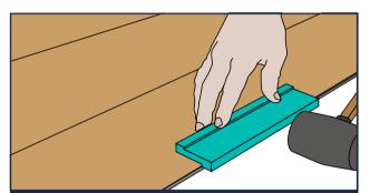
9. Continue to lay pieces along the second row by locking the long sides to the previous row. Gently tap the short edge joints with a soft rubber mallet to secure into place. Use a soft rubber mallet and a tapping block to make sure all joints are locked flush to one another.
