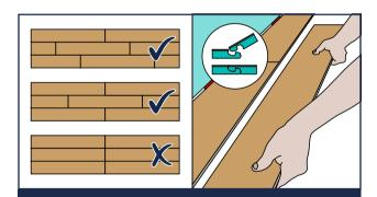
8. To attach the long edges, insert the long tongue side into the long groove side of the previous piece at an angle of around 30°. Gently apply inwards and downwards pressure until the joint closes, ensure that the short end joints are accurately aligned. The Plank can then be pushed / tapped flat to lock the joints into place. Always ensure the joints are staggered by at least a third.
