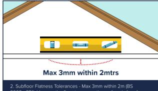
2003 - SR1). Vacuum the floor to ensure the surface is free from debris. Can be used with In-floor Radiant underfloor heating. Source must be min 13mm below flooring. Max Operating floor temperature 29°C refer to instruction manual.
