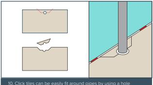
10. Click tiles can be easily fit around pipes by using a hole saw. Use a utility knife and cut a few centimeters away from the hole horizontally then at a 45° angle to the edge. Always leave a minimum expansion joint of 6-10mm around all pipes and objects. Reattach the pieces together using a vinyl seam sealer and wipe away any excess glue with a damp cloth.
