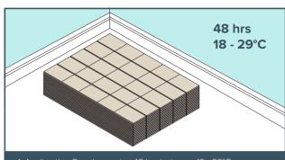
1. Acclimation Requirements - 48 hrs between 18 - 29°C. Check flooring for any damages to the tile or jointing lips. Dispose of damaged tiles. Read Instruction manual supplied in the box for preparation and in depth advise. Ensure that you plan out the cuts for both the width and length of your room. The final rows should be at least 1/3 of the width/length of the tile. If this is too narrow cut down the starting row width to ensure a reasonable width is achieved better stability.
