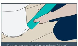
11. For splash areas such as bathrooms, waterproof skirting/scotia/trims can be used. Cut the flooring around your WC base leaving a 6-10mm expansion joint. 100% silicone sealant can be used around the expansion gap of a WC or small wet areas (sink pedestall), but cannot be used in large areas as this will restrict the expansion and contraction of the tiles and cause the joints to fail.
